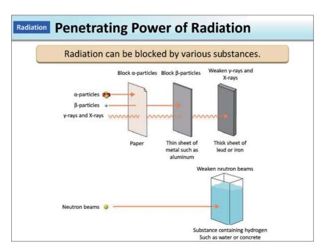
Charged particles or electromagnetic waves interact with a substance, lose their energy (speed), and eventually stop.
