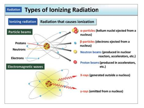
Particle beams include  $\alpha$  (alpha)-particles,  $\beta$  (beta)-particles, neutron beams, etc.
