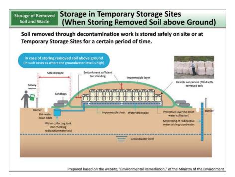
The soil and waste removed through decontamination work are stored and managed temporarily on site or at Temporary Storage Sites.
