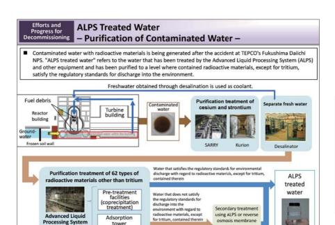
Contaminated water with radioactive materials is being generated after the accident at Tokyo Electric Power Company (TEPCO)'s Fukushima Daiichi NPS. "ALPS treated water" refers to the water that has been treated by the Advanced Liquid Processing System (ALPS) and other equipment and has been purified repeatedly to a level where contaminated radioactive materials, except for tritium, satisfy the regulatory standards for discharge into the environment.
