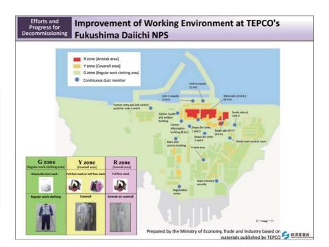
In order to improve safety and workability by reducing workers' load, efforts to improve the working environment, for such work as debris removal and paving of roads, have been made at Tokyo Electric Power Company (TEPCO)'s Fukushima Daiichi NPS. As a result, areas where workers can work in regular work clothing expanded to approx. 96% of the entire premises in June 2018.
