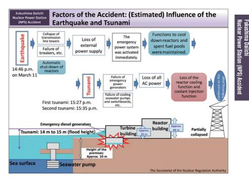
Immediately after the earthquake, at Units 1, 2 and 3 at Tokyo Electric Power Company (TEPCO)'s Fukushima Daiichi NPS, which were in operation, all reactors were shut down automatically.
