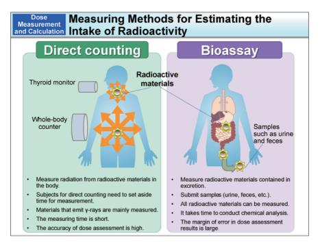
Direct counting methods that directly measure  $\gamma$ -rays coming from within the body or bioassay methods that measure the amount of radioactive materials in samples such as urine and feces are used to estimate the intake of radioactive materials, which is required for calculating internal exposure doses.
