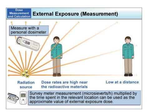
One of the means to measure doses due to external exposure is to wear a personal dosimeter on the body. Personal dosimeters can measure cumulative amounts of radiation exposure for a certain period of time, and provide dose rate readings.
