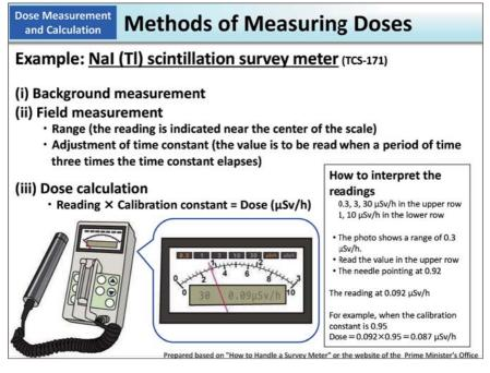
A method of measuring  $\gamma$ -ray ambient dose rate using a Nal scintillation survey meter is shown as an example of a method of measuring doses.
