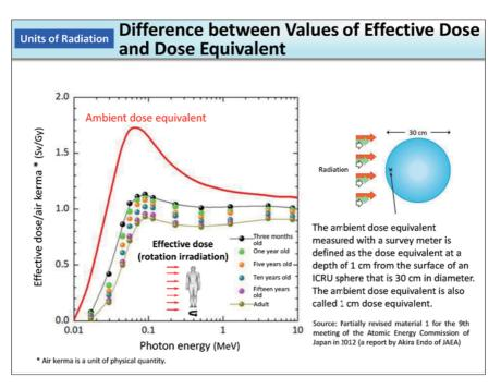
The ambient dose equivalent measured with a survey meter is set to always indicate a larger value than the effective dose.
