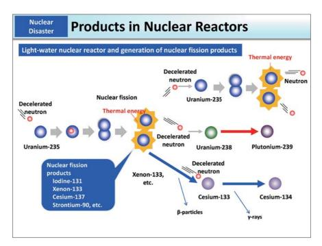
The light-water nuclear reactor is currently the most widely used type of reactor around the world (also used at Tokyo Electric Power Company (TEPCO)'s Fukushima Daiichi NPS). Bombarding enriched uranium fuel (Uranium-235: 3-5%; Uranium-238: 95-97%) with neutrons results in nuclear fission. Radioactive nuclear fission products such as Iodine-131, Cesium-137, and Strontium-90 are created in this process. When Uranium-238 is bombarded with neutrons. Plutonium-239 is created.
