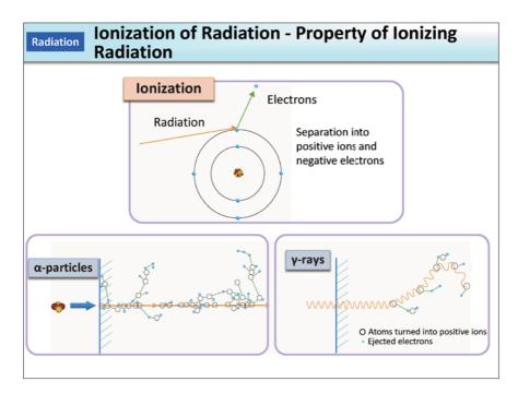
When radiation passes through a substance, its energy causes ejection of orbital electrons of the atoms that make up the substance, separating the atoms into positively charged atoms (or positive ion molecules) and free electrons. This is called ionization.
