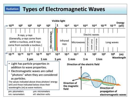
Electromagnetic waves are waves that propagate through space while an electric field and a magnetic field interact with each other. The shorter the wavelength is (the higher the frequency is), the higher the energy of an electromagnetic wave. The energy of radiation is expressed in electron volts (eV). 1 eV equals 1.6 x 10<sup>-19</sup> Joule (J).
