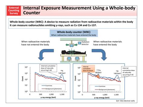
A whole-body counter is a device to measure  $\gamma$ -rays emitted from the body. As  $\gamma$ -ray energy differs by radionuclide, if a specific amount of energy, for example, 1,461 keV, which is the  $\gamma$ -ray energy of radioactive potassium (K-40), is counted, this can be interpreted as  $\gamma$ -rays emitted from K-40 in the body. The  $\gamma$ -ray energy of Cs-137 is 662 keV.
