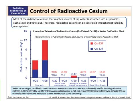
As of April 2011, radioactive cesium concentrations in raw water, water after sedimentation, biological activated carbon treated water, and rapid filtered water were measured at water purification plants in Fukushima Prefecture. As a result, it was confirmed that low-concentrated radioactive cesium detected in raw water had decreased through adsorption into soil in the process of sedimentation.
