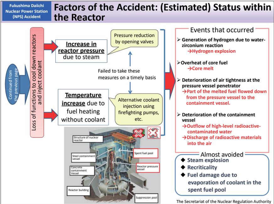
As coolant injection to the reactor core was suspended, the water level in the reactor declined and the fuel was exposed. This caused core melt and damaged the pressure vessel. Additionally, under high temperature due to core damage, steam and zirconium of the fuel clad reacted to generate a large amount of hydrogen, which was released within the containment vessel together with steam.
