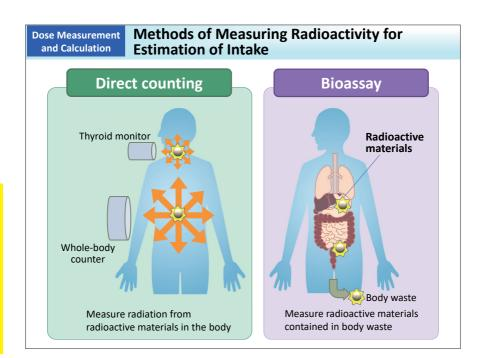
Direct counting methods that directly measure  $\gamma$ -rays coming from within the body or bioassay methods that measure the amount of radioactive materials in urine or feces are used to estimate the intake, which is required for calculating internal exposure doses.
