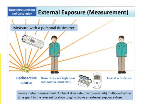
Wearing a personal dosimeter on the body is one of the means to measure doses due to external exposure. Personal dosimeters can measure cumulative amounts of radiation exposure for an extended period of time, and provide hourly readings.
