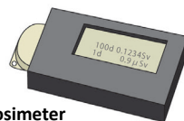
Electronic Personal Dosimeter Equipped with a device to display dose rates or cumulative doses during a certain period of time and thus convenient for measuring and managing exposure doses of temporary visitors to radiation handling facilities
