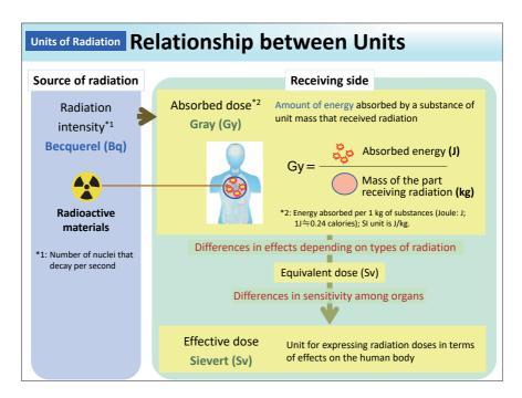
Units of radiation can be broadly divided into units for sources of radiation and units for the receiving side. Becquerel, a unit of radioactivity, is used for sources of radiation. Units for the receiving side are gray and sievert.
