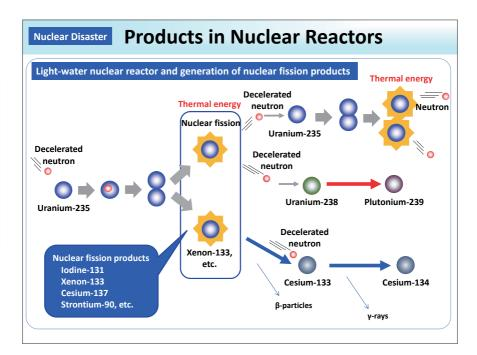
The light-water nuclear reactor is currently the most widely used type of reactor around the world (also used at Tokyo Electric Power Company (TEPCO)'s Fukushima Daiichi NPS). Bombarding enriched uranium fuel (Uranium-235: 3-5%; Uranium-238: 95-97%) with neutrons results in nuclear fission. Radioactive nuclear fission products such as Iodine-131, Cesium-137, and Strontium-90 are created in this process. When Uranium-238 is bombarded with neutrons. Plutonium-239 is created.
