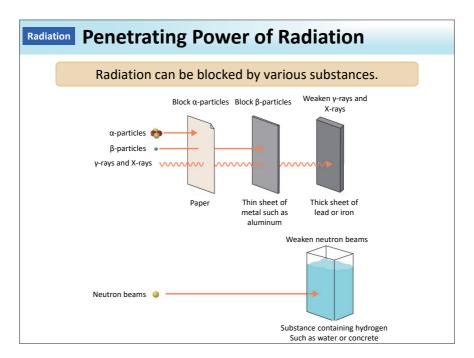
Charged particles or electromagnetic waves interact with a substance, lose their energy (speed), and eventually stop.
