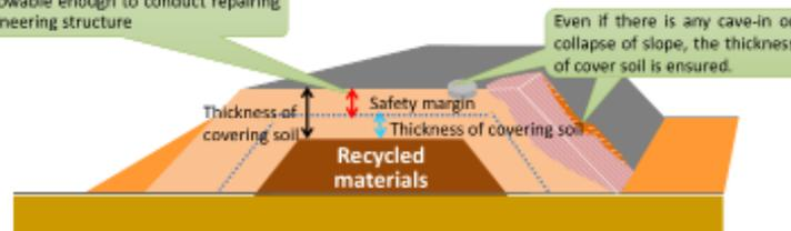
Covering soil should be designed to ensure the necessary thickness to confine the additional exposure dose, even under general repairing of a civil engineering structure.
