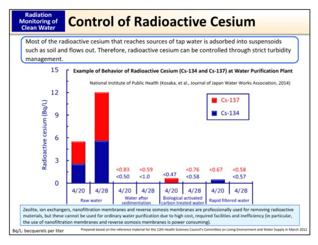
As of April 2011, radioactive cesium concentrations in raw water, water after sedimentation, biological activated carbon treated water, and rapid filtered water were measured at water purification plants in Fukushima Prefecture. As a result, it was confirmed that low-concentrated radioactive cesium detected in raw water had decreased through adsorption into soil in the process of sedimentation.
