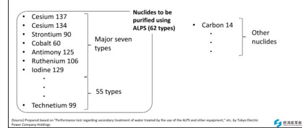
Contaminated water generated at Tokyo Electric Power Company (TEPCO)'s Fukushima Daiichi NPS contains not only tritium but also Cesium 137, Strontium 90, Iodine 129, and other radioactive materials. These types of radioactive materials normally remain in nuclear fuel rods at ordinary nuclear power stations and are seldom detected in water discharged therefrom. (Related to p.30 of Vol. 1, "Products in Nuclear Reactors")
