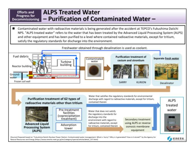
Contaminated water with radioactive materials is being generated after the accident at Tokyo Electric Power Company (TEPCO)'s Fukushima Daiichi NPS. "ALPS treated water" refers to the water that has been treated by the Advanced Liquid Processing System (ALPS) and other equipment and has been purified to a level where contaminated radioactive materials, except for tritium, satisfy the regulatory standards for discharge into the environment.
