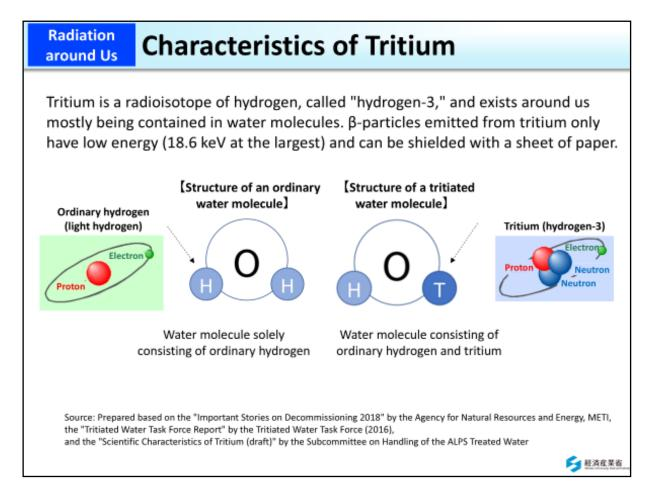
The water processed with the multi-nuclide removal equipment, also called the Advanced Liquid Processing System (ALPS), or other equipment, at Tokyo Electric Power Company (TEPCO)'s Fukushima Daiichi NPS, still contains tritium, which is a radioactive material.
