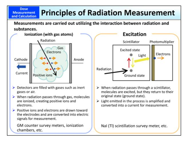
Radiation is known to interact with substances when passing through them. The amount of radiation can be measured utilizing the interaction between radiation and substances.
