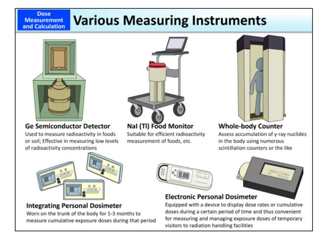
While radiation is not visible to the human eye, it is known to cause ionization and excitation (p.45 of Vol. 1, "Principles of Radiation Measurement"), and a variety of measuring instruments using these effects have been invented for different purposes and applications. The measuring instruments shown above all utilize the excitation effect.
