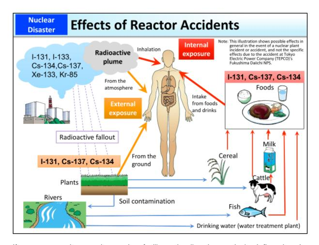
If an emergency happens in a nuclear facility and radioactive gas leaks, it flows into the atmosphere in a state called "plume." Plumes contain radioactive noble gases and aerosols (micro liquid droplets and particles), such as radioactive iodine and radioactive cesium.
