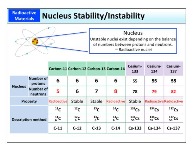
Nuclei having the same atomic number (the number of protons) but differing in the number of neutrons are called "isotopes" to each other. There are "radioisotopes" that emit radiation upon radioactive disintegration and "stable isotopes" that do not emit radiation and so do not change in atomic weight.
