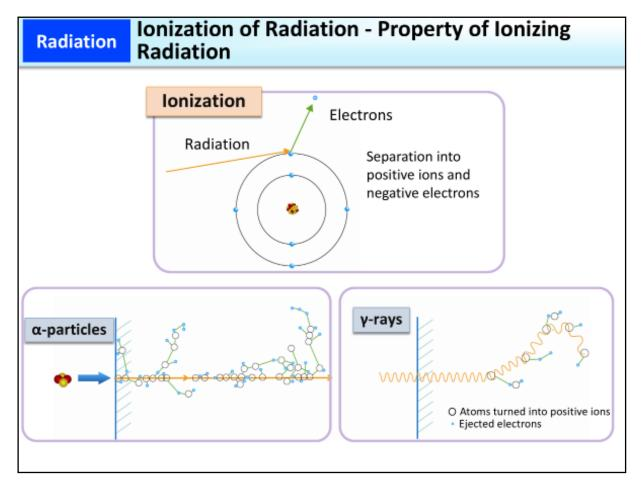
When radiation passes through a substance, its energy causes ejection of orbital electrons of the atoms that make up the substance, separating the atoms into positively charged atoms (or positive ion molecules) and free electrons. This is called ionization.
