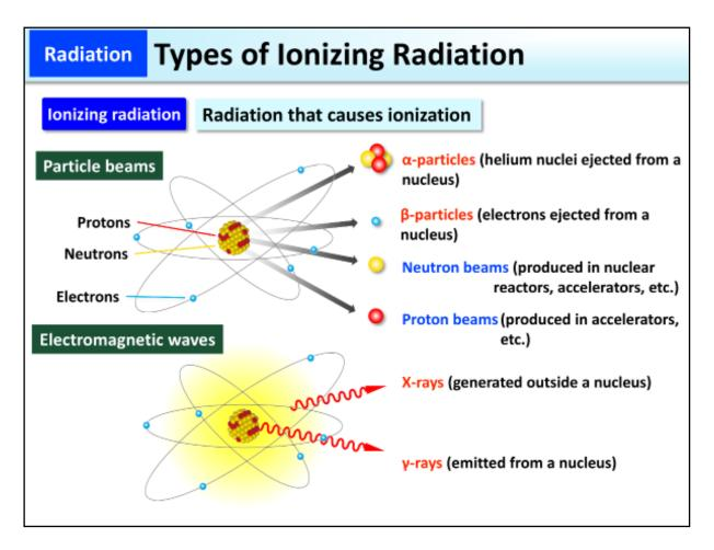
Particle beams include  $\alpha$  (alpha)-particles,  $\beta$  (beta)-particles, neutron beams, etc.
