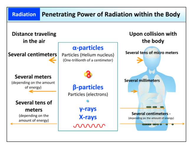
The easiness to penetrate through the air or the human body varies depending on the types of radiation. Therefore, the types of radiation ( $\alpha$  (alpha)-particles,  $\beta$  (beta)-particles, or  $\gamma$ -rays) and radioactive materials (nuclides) that cause problems differ for external exposure and internal exposure.
