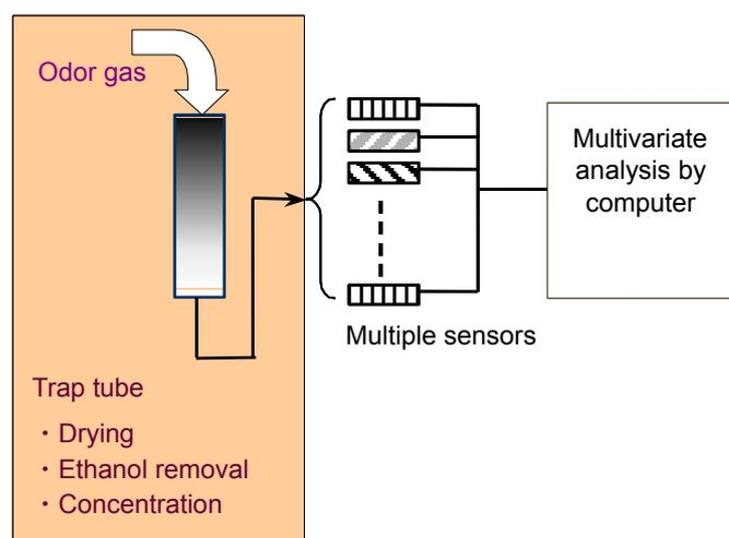
Fig. 4 Electronic Nose Configuration
