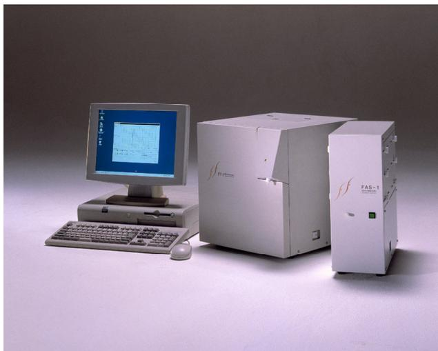
Fig. 5 Appearance of the Electronic Nose
