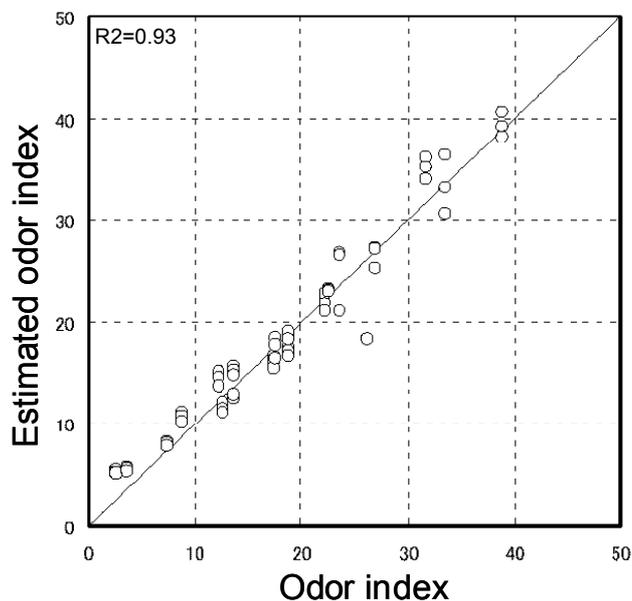
Fig. 7 Odor Intensity Prediction using Multiple Regression Analysis
