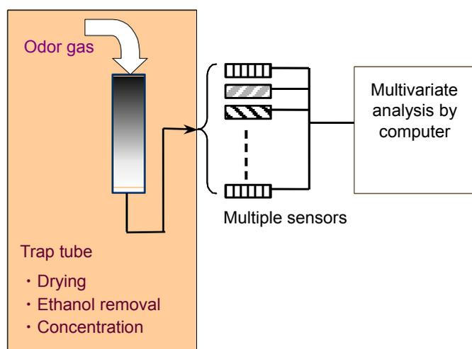
Fig. 4 Electronic Nose Configuration
