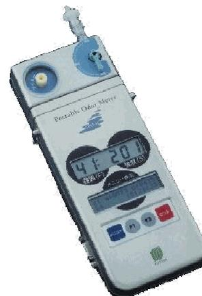
Fig.2 Odor Sensor with Two Sensor Elements
