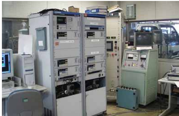
Figure 1-19 CO, HC, NO x , CO 2 measurement apparatus: exhaust gas analysis system
