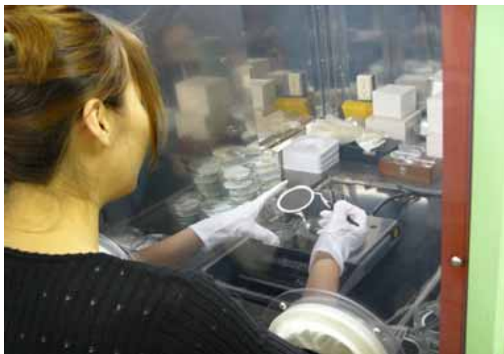
Figure 1-20 Weighing the particulate matter collected (weighing chamber)
