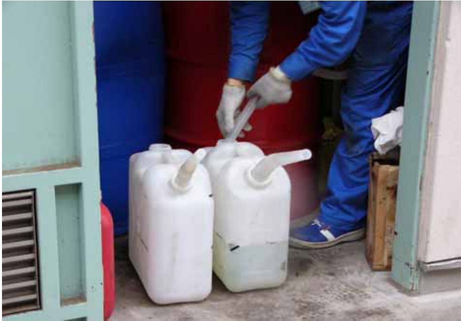
Figure 1-27 Mixing the blends of BDF and diesel fuel
