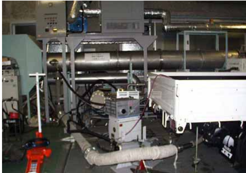
Figure 1-17 Measuring exhaust gases from test vehicle
