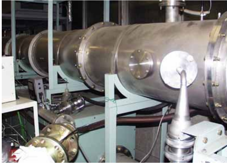
Figure 1-18 Exhaust gas/PM measurement apparatus: full dilution tunnel and part of PM collection filter
