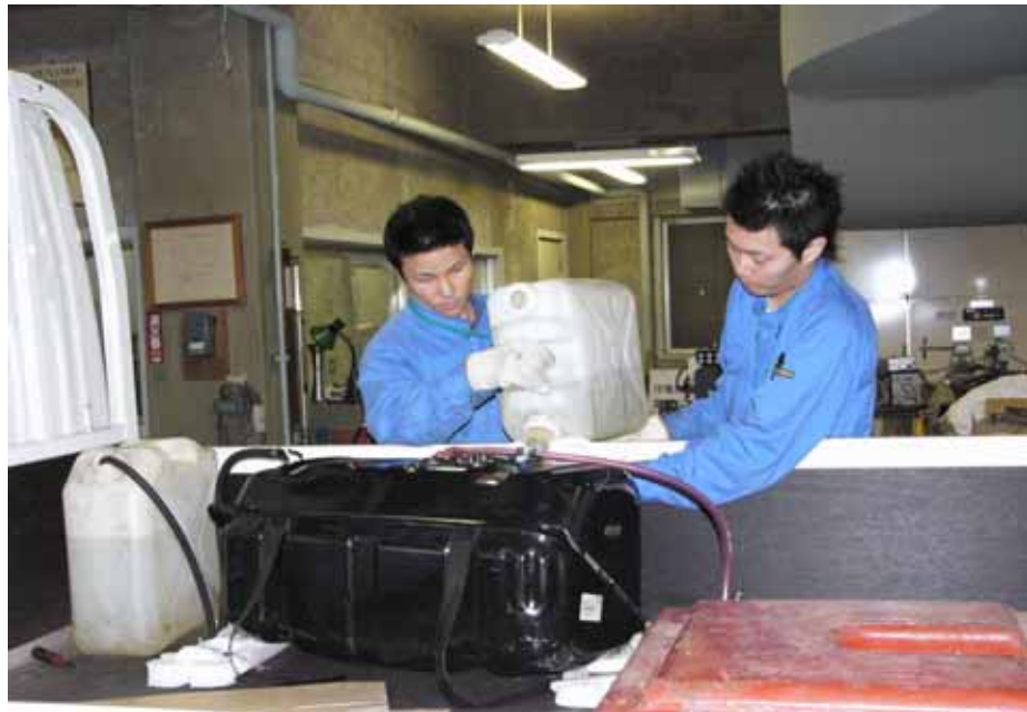
Figure 1-28 Filling the test fuel tank with a BDF and diesel fuel blend
