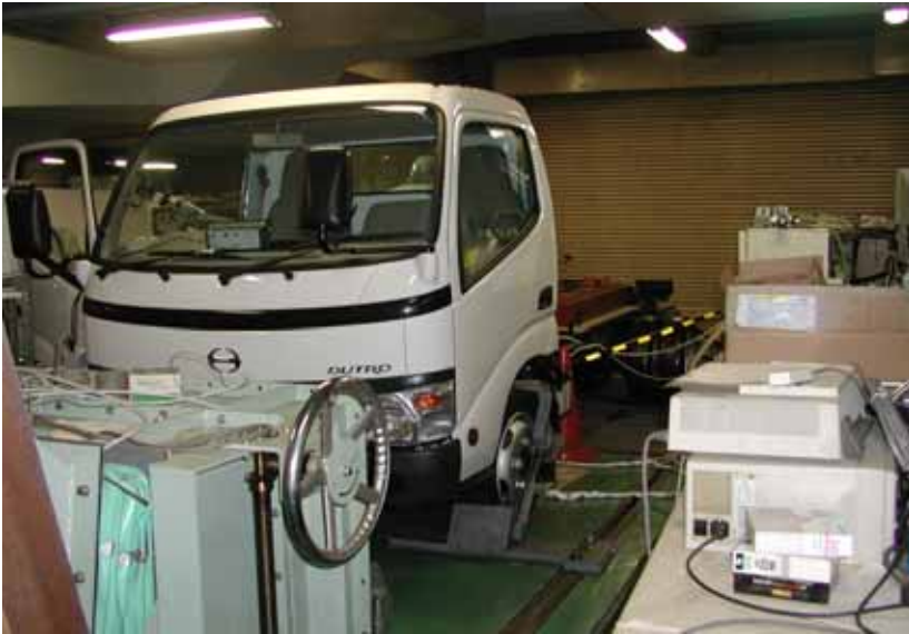
Figure 1-13 Vehicle C chassis dynamometer testing (from front)
