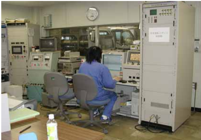
Figure 1-16 Chassis dynamometer control unit
