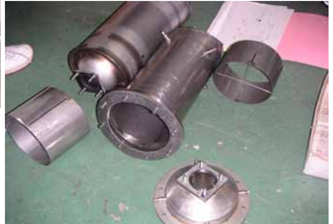
Figure 1-10 Container for catalyst replacement tests on Vehicle B
