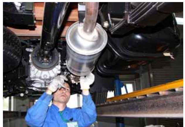
Figure 1-8 Replacing catalyst on Vehicle B
