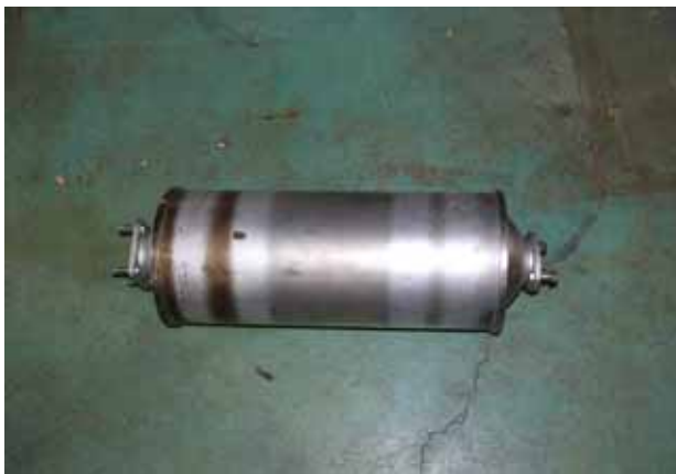
Figure 1-7 Catalyst fitted as standard on Vehicle B
