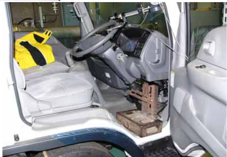
Figure 1-4 Vehicle A steady state testing (jig fixing accelerator pedal)
