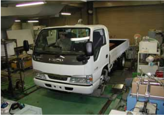
Figure 1-5 Vehicle B chassis dynamometer testing (from front)
