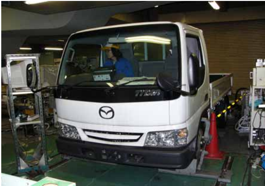
Figure 1-2 Vehicle A chassis dynamometer testing
