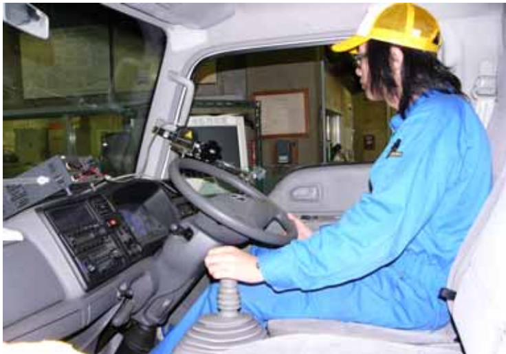
Figure 1-2 Vehicle A chassis dynamometer testing
