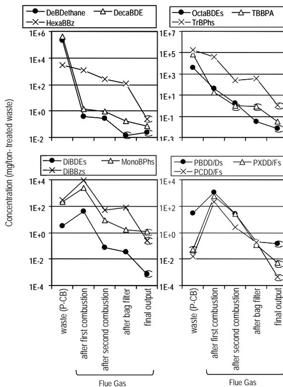
Fig. 6. Behavior of BFRs and dioxin related compounds during waste combustion and flue gas treatment processes (the symbols in parenthesis are below the detection limits).
