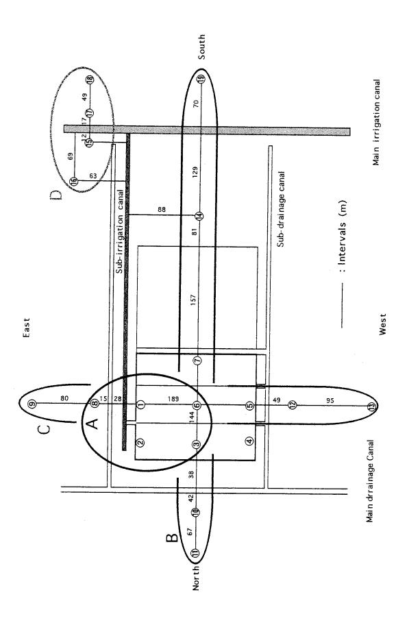
Fig.  ${f 2}$  Observation sites shown in circled number for measuring grondwater levels and water quality in and around the experiment field
