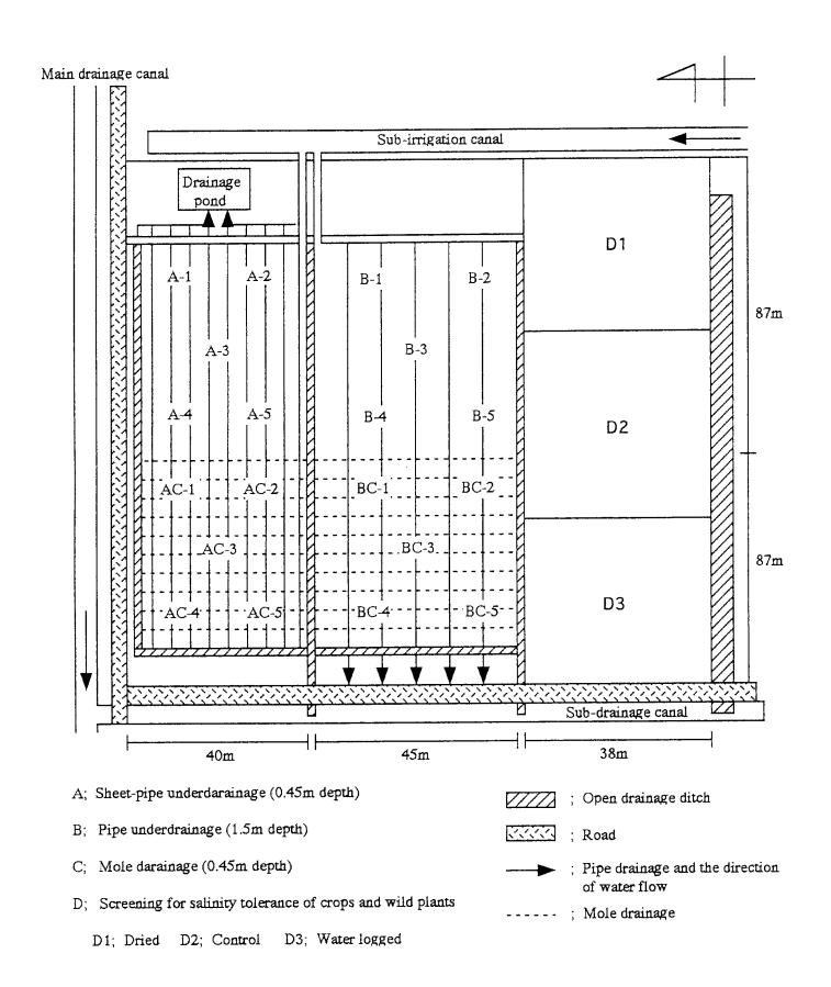
Fig. 1 Field layout of drainage treatments and soil sampling sites
