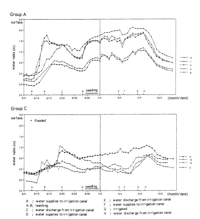
Fig.  $\bf 3$  Time-course changes of water table in and around the experiment fields under irrigated conditions
