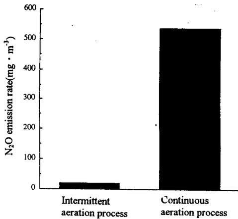
Fig.5 N<sub>2</sub>O emission rate per 1m<sup>3</sup> of treated sewage
