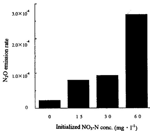
Fig. 3 N<sub>2</sub>O emission rate per 1mg of MLSS
