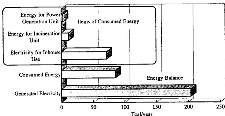
Fig.8 Energy balance around an incineration system for municipal waste with power generation plants
