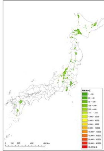
Figure 14 Low-temperature binary power generation introduction potential distribution chart (53 to 120°C or more, basic)
