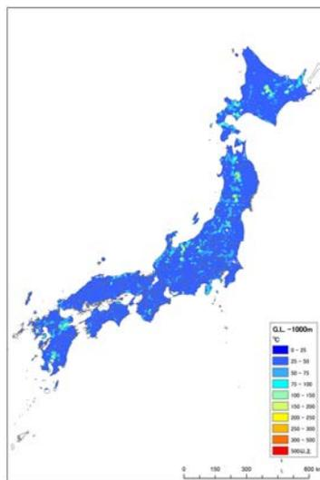
Figure 2 Underground temperature structure data (G.L. -1000 m)
