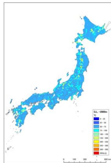
Figure 3 Underground temperature structure data (G.L. -2000 m)
