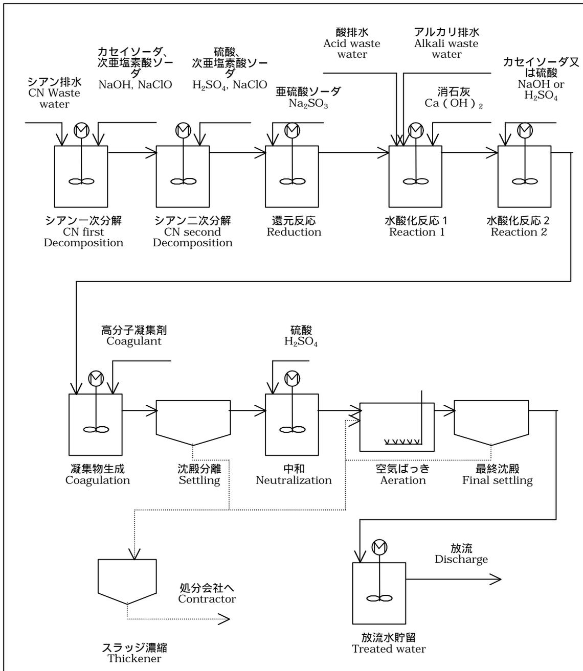
For the removal of such heavy metals as iron, nickel and copper, the solution is again made alkaline with the pH value of around 10 by the addition of slaked lime, Ca(OH)<sub>2</sub>, to convert these heavy metals into water-insoluble hydroxides. Then, a polymer coagulant is added to form large flocs out of metal hydroxides to let them sediment in the setting basin. The polymer coagulant is purchased from a Japanese water treating equipment manufacturer.
