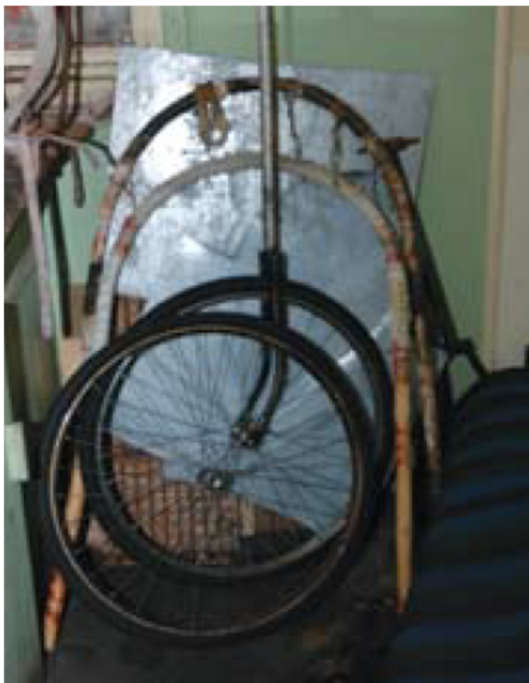
Bicycle wheels used to make sledge meters to measure the distance run
