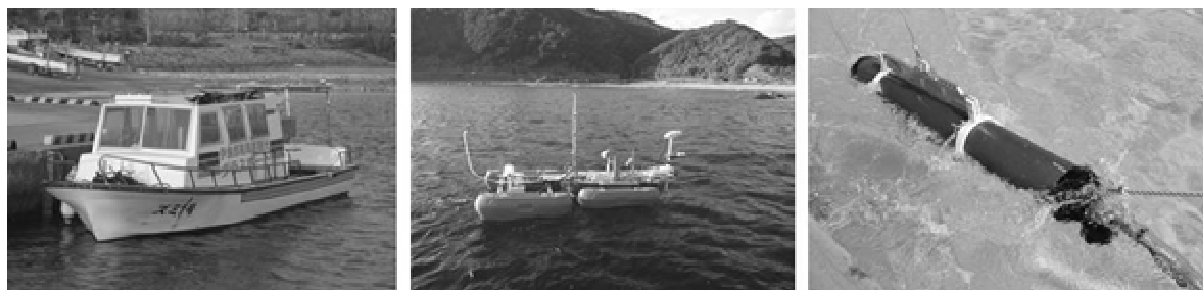
Fig. 1: Photographs of the boat-based coral observations. (left) the glass-bottom-boat based fluorescence imaging lidar system (center) the autonomous self-propelled mini boat-based stereoscopic-imagery system (right) the towed buoy-based fluorescence imaging lidar system
