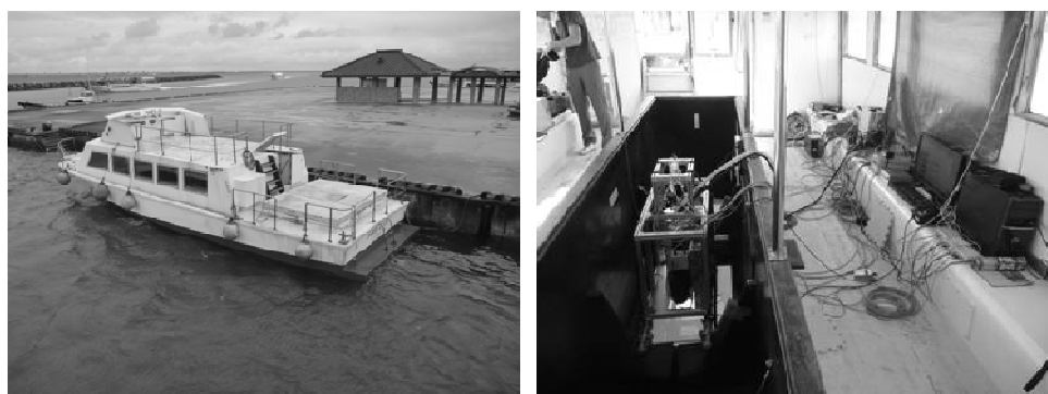
Figure5 The glass-bottom-boat at Taketomi island, Okinawa (left) and the overview of the imaging fluorescence lidar system installed on the glass-bottom-boat (right)
