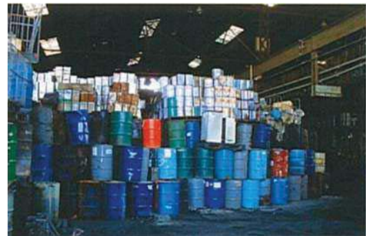
Improper disposal (excessive storage amount)
