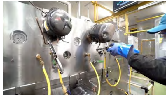
Recovery of CFC gas from compressors
