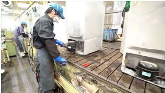
Hand disassembly of refrigerator
