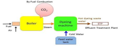
Figure 5 A Situation without Waste Heat Recovery
