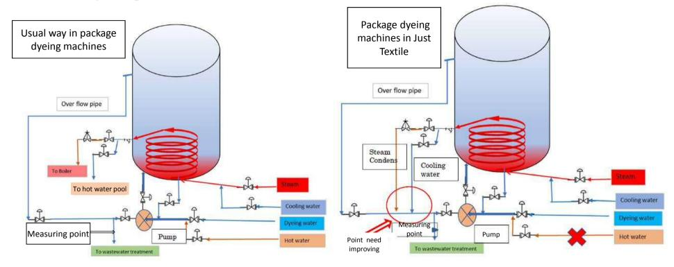
☐ It is important to separate pipes for collecting steam condense, cooling water and waste water to recover waste heat efficiently.
