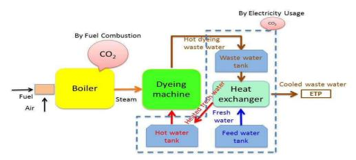
Figure 6 A Case of Introduction of Waste Heat Recovery
