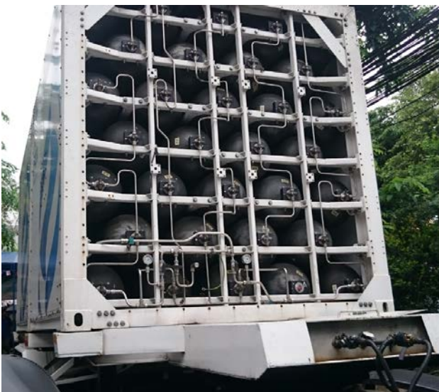
Mobile Refueling Unit (MRU) の内部
