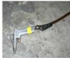
point: air gun 49. 2L/min
