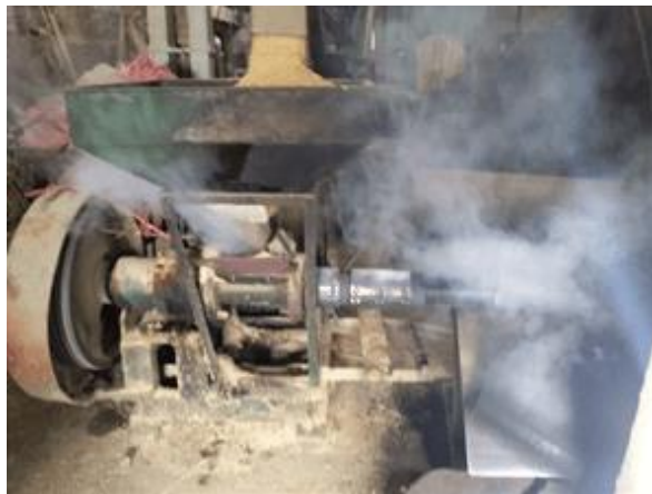
Figure22 Local briquette machine with a hopper (Rice husks are fed from the top)
