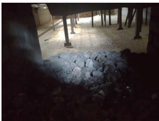
Figure52 Coal inlet to the combustion furnace (Combustion gases enter the lower part of the drying chamber.)
