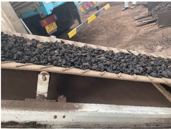
Figure74 Coal is being fed to furnace for combustion
