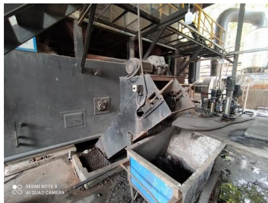
Figure70 Discharge system for furnace bottom slag
