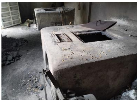
Figure51 Coal feed port to the combustion furnace (left), coal placed in the coal combustion furnace (right)
