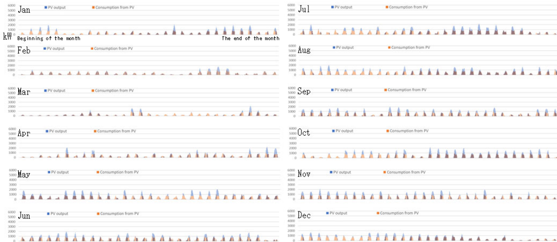
Figure 2.2.6.1.1. Variations in the amount of electricity generated by a system with a PV capacity of 3 MWp over 365 days.
